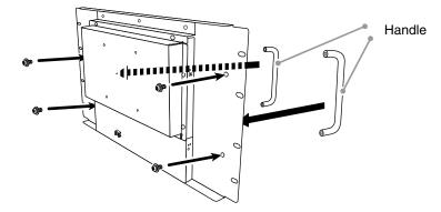
2. Attach the monitor to the rack while holding the handles on both sides and then secure the monitor using screws.
