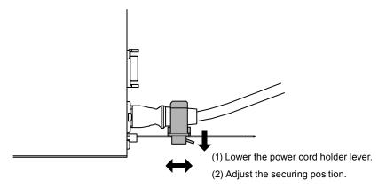
3. Secure the power cord holder to prevent the power cord from falling off.
