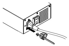
2. Adjust the position to secure the power cord holder referring to the figure shown below.
