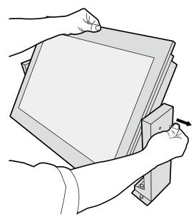
**2.** Adjust the angle and secure the monitor using the tilt lock pin.
