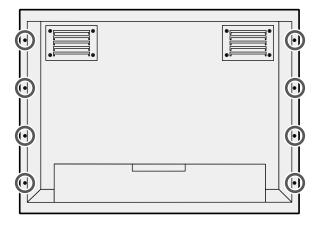
2. Fasten one of the stands by screwing the included screws and bolts into the seven screw holes in the back panel of the monitor.
