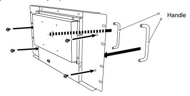
2. Attach the monitor to the rack while holding the handles on both sides and then secure the monitor using screws.
