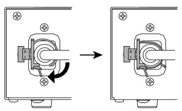
\*Check that the power cord holder is secured.
