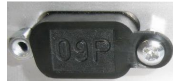
Fig. 11: ESD protection cover for the male serial port
