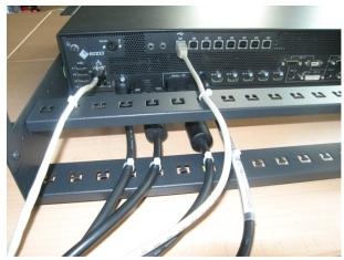
Cable ties, 3 mm in width, can be used to attach the cables.
