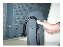
8. Route the connecting cable in the cable duct.
