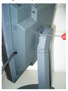
7. Then carefully turn the monitor  $90^{\circ}$  clockwise and tighten the lower screws.
