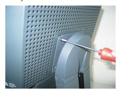
6. First tighten the top two screws.
