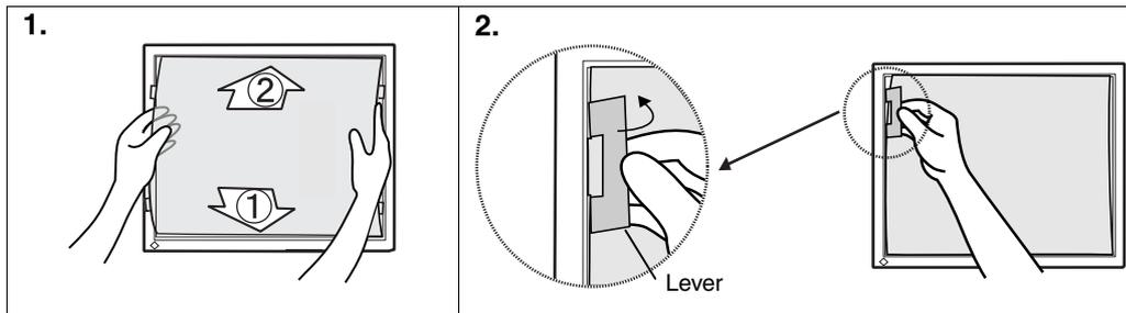
1. Set the panel protector into the grooves of the panel frame; the lower first (1), then the upper (2).
