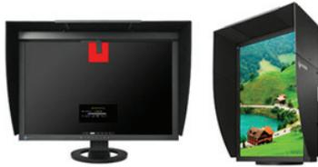
Designed for pre-press, digital photography, video editing, and post production work, this 24.1" LCD monitor houses a built-in calibration device in its upper bezel that swings down at user-scheduled times. This eliminates the need for a third party external calibration device which must be manually placed over the monitor's screen and then removed again every time calibration is performed.
