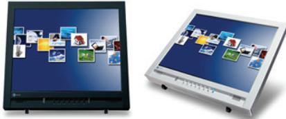
17-inch FlexScan T1751 LCD monitor. The FlexScan T1751 offers multitouch capabilities through Windows 7 for an intuitive way to use applications with two fingers on the screen by tapping, scrolling, dragging, pinching, etc.
