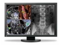
screen size and native resolution of 4 megapixels ( $2560 \times 1600$ ) for a 16:10 widescreen format give this monitor the same amount of screen size and number of pixels as two 2 megapixel monitors in portrait mode but without the obtrusive bezels. This simplifies comparing images or allows for showing more information – for example 12 computed tomography slices with an information volume of 512 × 512 pixels each.
