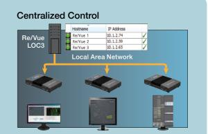
Re/Vue products can be managed through the Lights Out Configuration 3 (LOC3) utility that provides access to settings and controls for flexible management of the network from a centralized location. It also lets you set the display orientation to landscape or portrait mode so that the video is streamed in the correct format.
