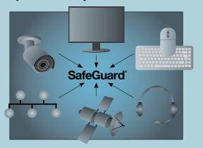
SafeGuard supports the capture of audio (analog, digital, VoIP), radar (serial or network), keyboard and mouse, At-the-Glass video signals (analog and digital), CCTV camera signals, and distributed network data. Synchronous data playback is achieved through the selection of multiple channels of varying types from a user-specified timeframe.
