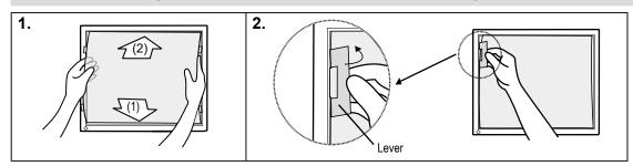
1. Set the panel protector into the grooves of the panel frame; the lower first (1), then the upper (2).
