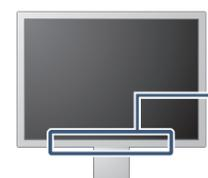
1. Press the power button to turn on the monitor.
