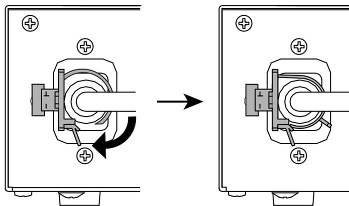
\*Check that the power cord holder is secured.
