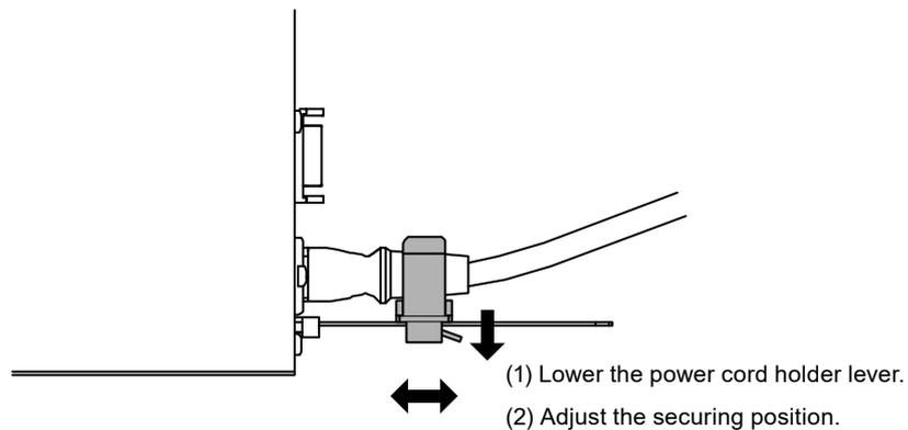
3. Secure the power cord holder to prevent the power cord from falling off.
