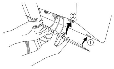
Example: Installing the Cable Cover (Right)
