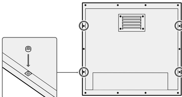
2. Fasten one of the stands by screwing the included screws into the two screw holes where the spacers have been inserted.
