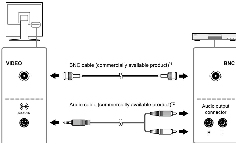
\*1 If the video output connector for the analog video equipment has an RCA plug, use a commercially available BNC-RCA conversion adapter to make the connection.
