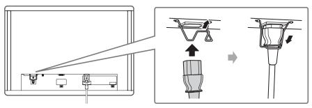
5. Connect the power cord to a power outlet.
