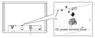
2. Strip the wire insulation (strip length: 7 mm  $\pm$  0.5 mm). If tip treatment is required, attach a rod terminal (ferrule). Use ferrules made by Phoenix Contact.
