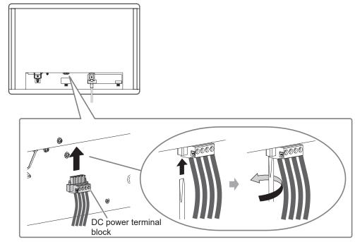
5. Fasten with a cable tie so that the cables do not come off.
