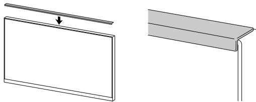
4. Install the edge support at the aligned position while ensuring that there are no gaps between the LCD panel surface and the edge support.
