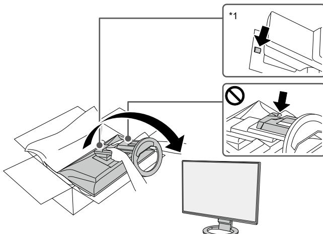
\*1 The lock button is only used to remove the stand from the monitor.
