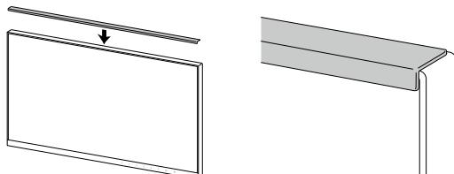
5. Install the edge support at the aligned position while ensuring that there are no gaps between the LCD panel surface and the edge support.
