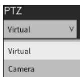
Virtual: Performs the PTZ operation by digitally processing the camera images inside the product.
