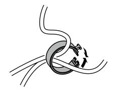
3. While holding the cable holder closed, attach it onto the stand.
