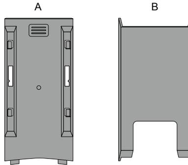
1. Align the tabs of (A) with the attachment parts of the stand.
