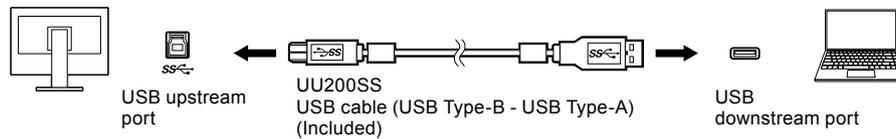
2. Connect a peripheral USB device to the USB downstream port of the monitor.
