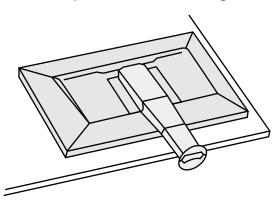
2. Attach the stand base onto the stand brace.
