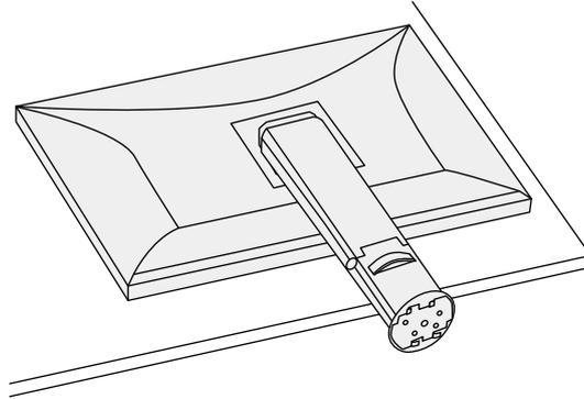
2. Hold the stand base so that the back label ( **FRONT** ) is aligned as shown in the diagram, and attach the stand base onto the stand brace.
