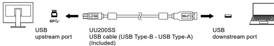
2. Connect a peripheral USB device to the USB downstream port ([page 9](#)) of the monitor.
