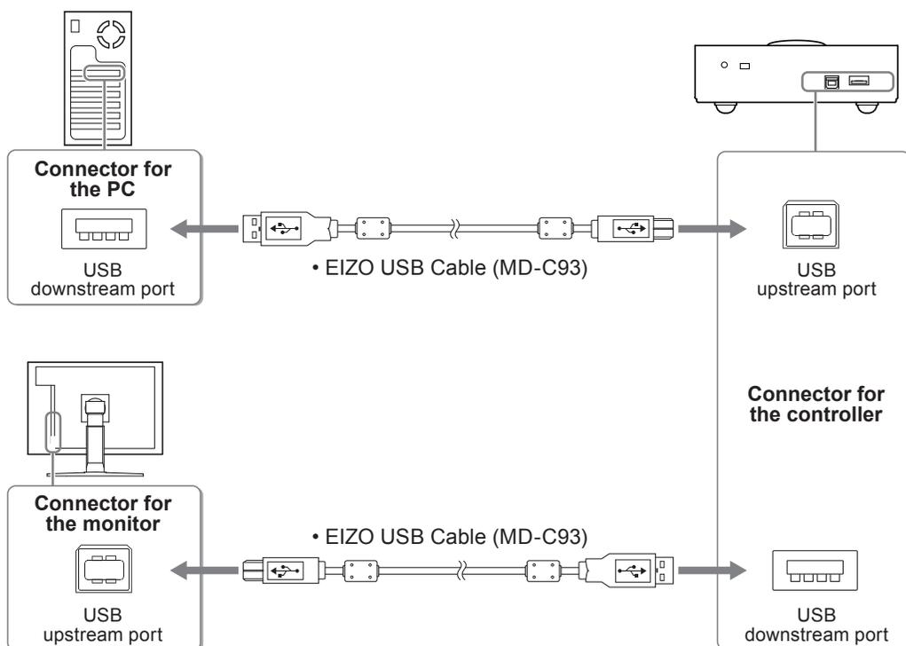
When the connection is completed, the ENTER button lights in blue.
