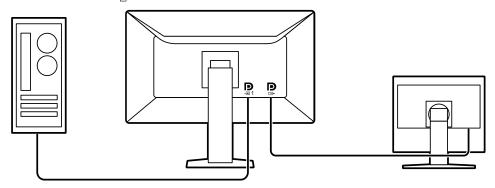
• In order to display images in PbyP, two signal cables usually need to be connected between the PC and the monitor. On this model, you can connect it to the PC using one cable. You only need to connect the supplied DisplayPort cable (PP028) between the output terminal ( ) and the input terminal ( ).
