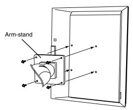
4 Mounting Screws: M4  $\times$  10 (mm) Ni/Fe
