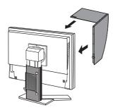
(2) Insert the hook into the hole\* on the hood (a) and slide it down along the projection on the back side of the monitor (b).
