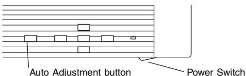
The ScreenManager operation can be disabled by holding down the Auto adjustment button while switching on the LCD monitor's power. This will disable (“lock”) the Enter button and Auto adjustment button, protecting from accidental changes. To unlock the buttons, switch the power off. Switch the power on while pressing the Auto adjustment button.
